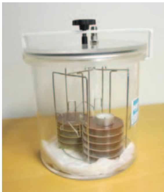
Figure 4.3 Candle extinction jar for incubation of N. gonorrhoeae culture plates
